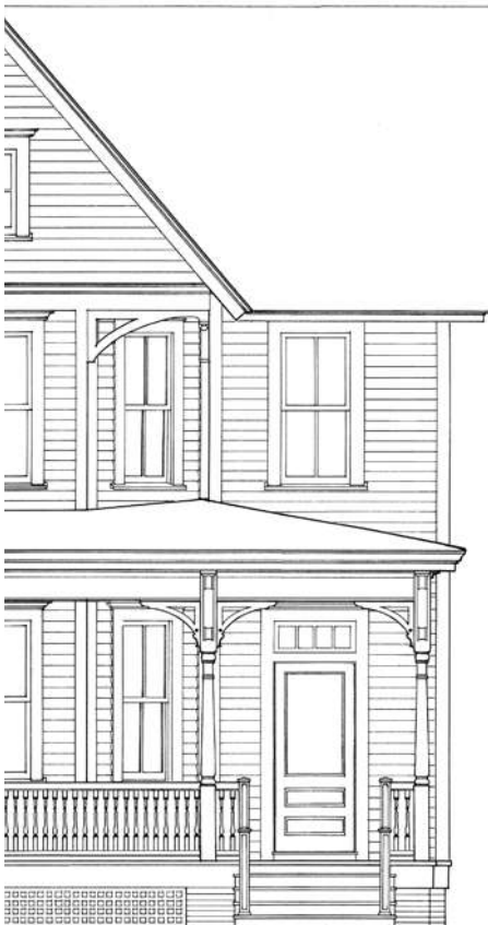
One-story, hipped porch partial elevation
